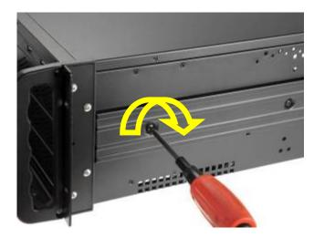
2. Unscrew all three screws on each side.
